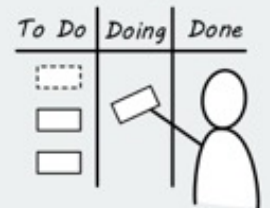
Pull system for work
